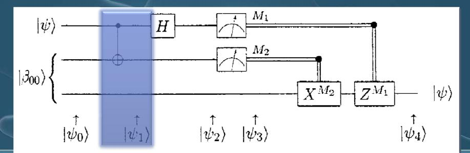
$$\begin{aligned} U_{H} &= \binom{1}{1} & \frac{1}{-1} \big) / \sqrt{2} \otimes \begin{pmatrix} 1 & 0 & 0 & 0 \\ 0 & 1 & 0 & 0 \\ 0 & 0 & 1 & 0 \\ 0 & 0 & 0 & 1 \end{pmatrix} \\ \rho_{2} &= U_{H}^{\dagger} \cdot \rho_{1} \cdot U_{H} \end{aligned}$$
